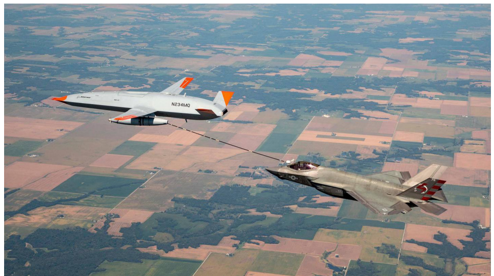
An MQ-25 test asset conducts its first aerial refueling test flight with an F-35C Lightning II on Sept. 13, 2021, near the MidAmerica St. Louis Airport in Illinois. (Boeing)
