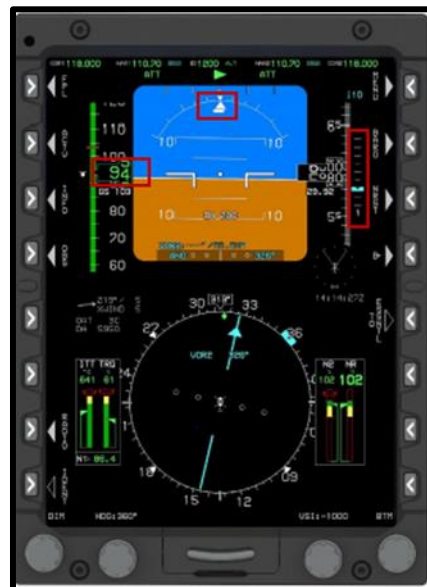
Figure 2-3 Rate Instruments (Airspeed, Turn and Slip Indicator, VSI)
