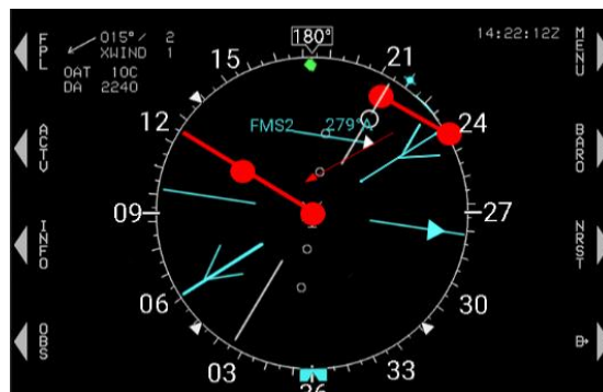
Figure 3-6 HSI Point-to-Point Flying from 240 Radial at 10 DME to 210 Radial at 8 DME
