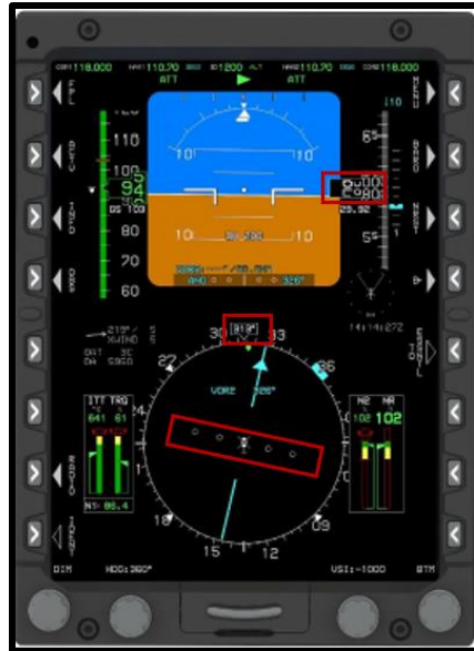
Figure 2-2 Position Instruments (Altimeter, Heading Indicator, HSI)
