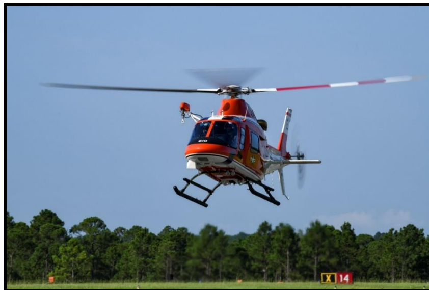
Figure 3-7 TH-73A with Hoist Installed
