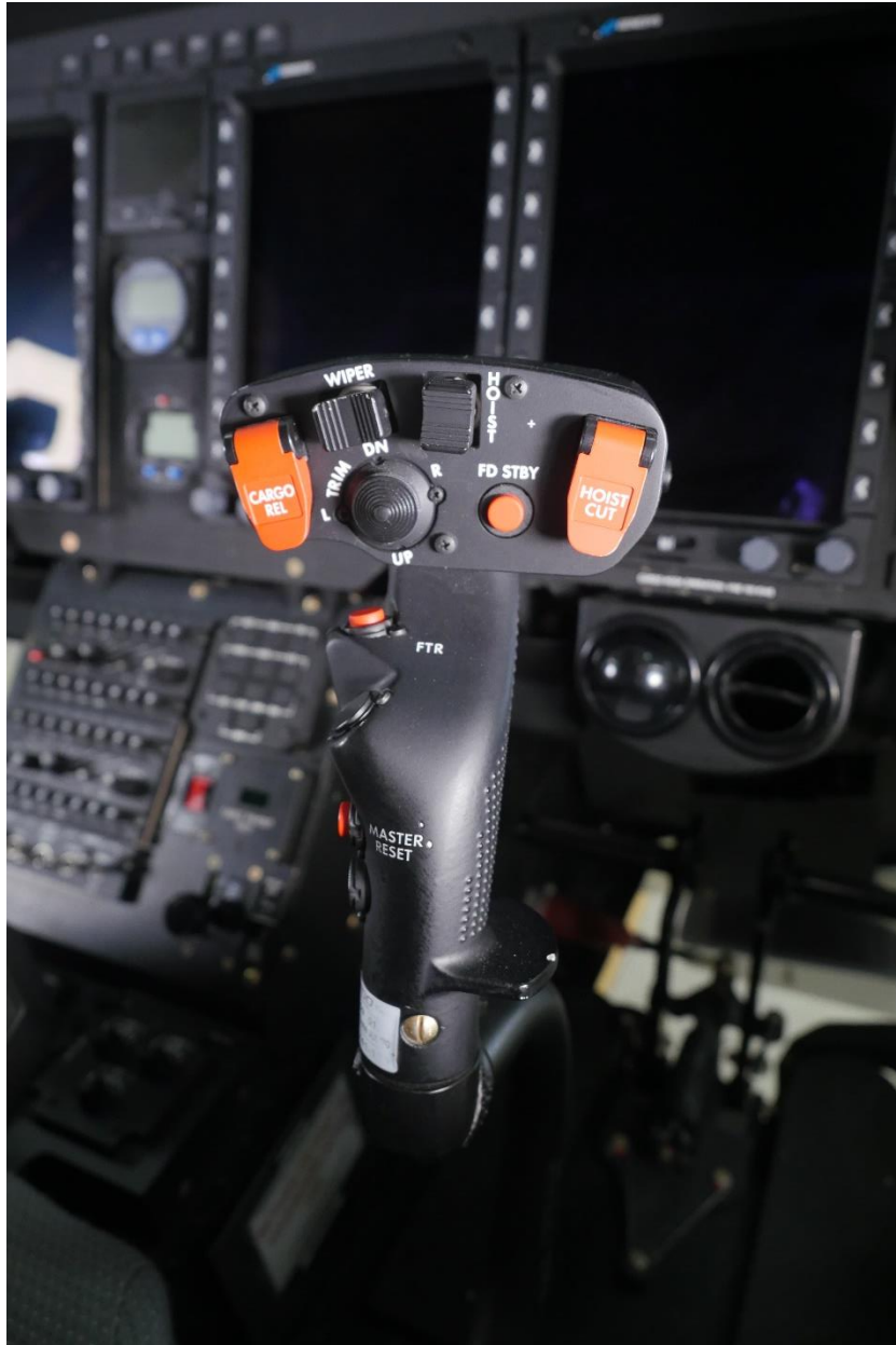
Figure 3-9 Hoist Control Switch on Cyclic
