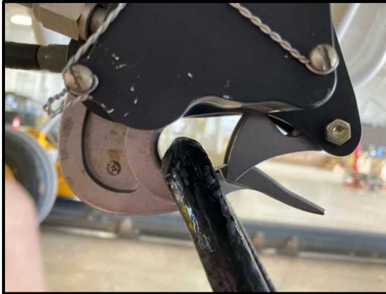
Figure 3-2 DSG 12-4K Pendant Attached to TH-73A Cargo Hook
