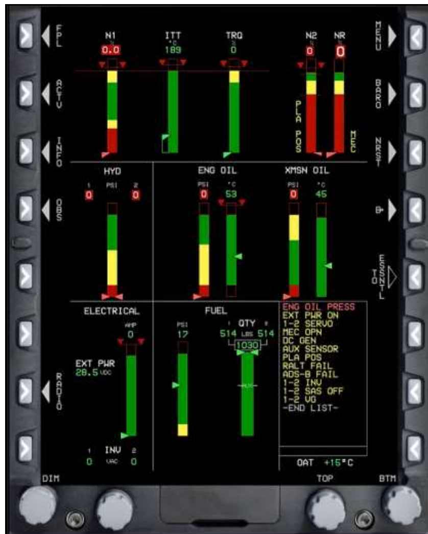
Figure 1-2 Normal Indications Prior to Engine Start While on External Power
