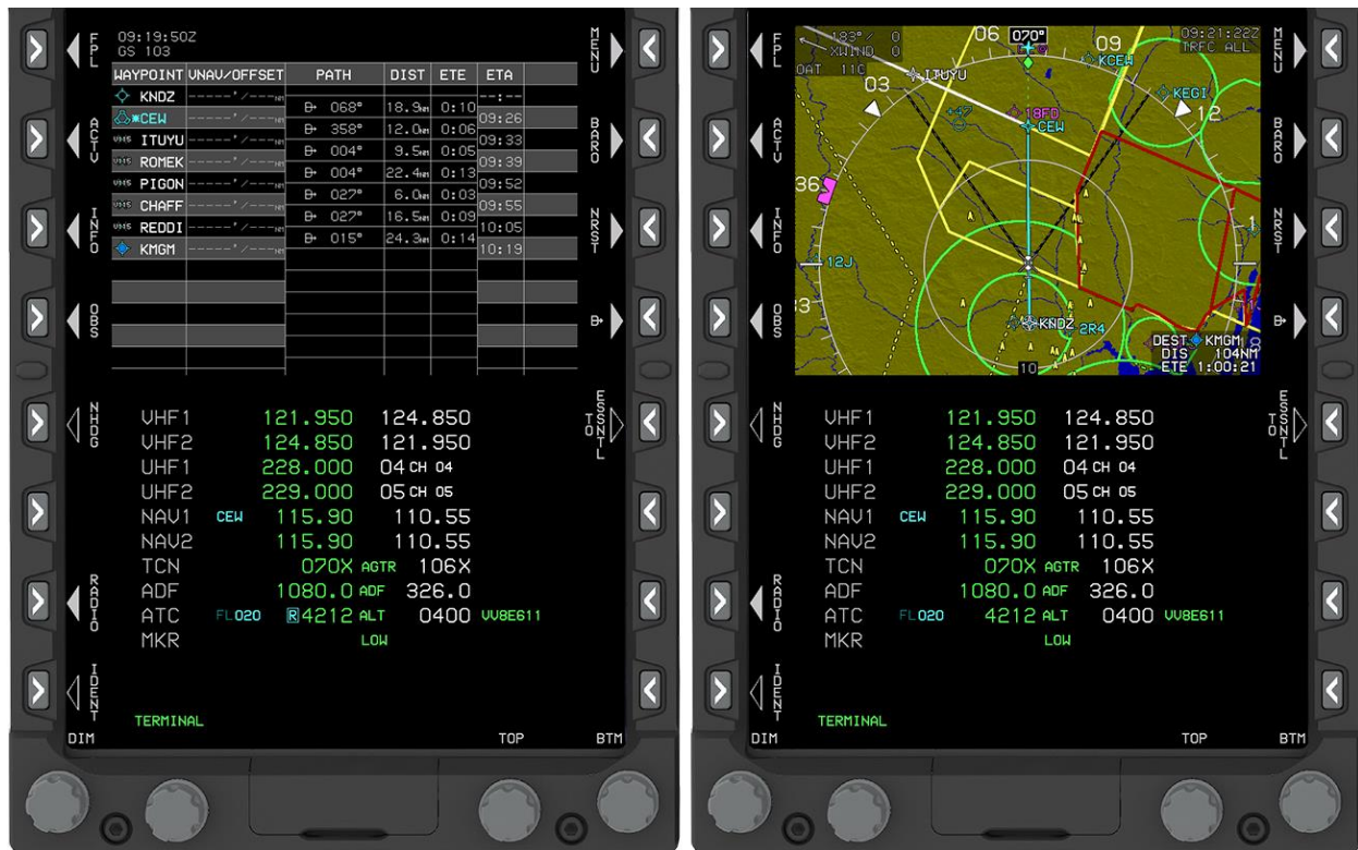
Figure 1-5 Verify the Flight Plan by Viewing NAV LOG or MAP on the MFD
