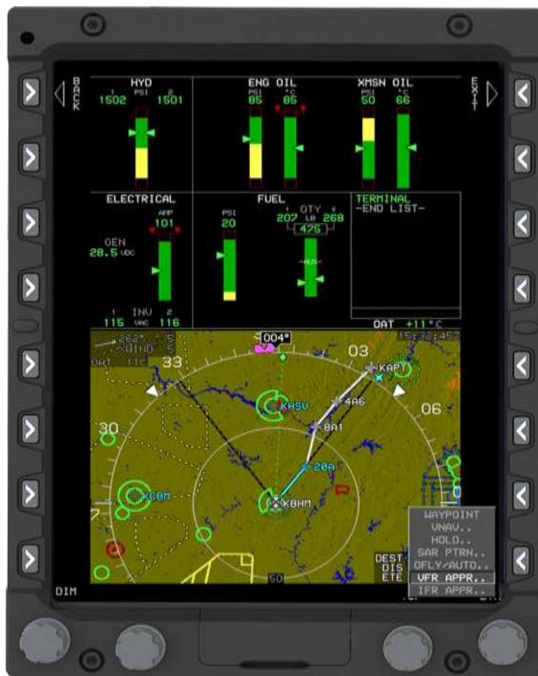
Figure 3-3 VFR APPR on the Flight Plan Menu
