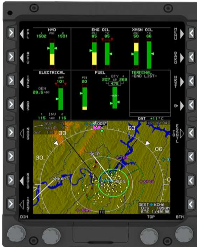
Figure 3-4 Approach Added to a Flight Plan
