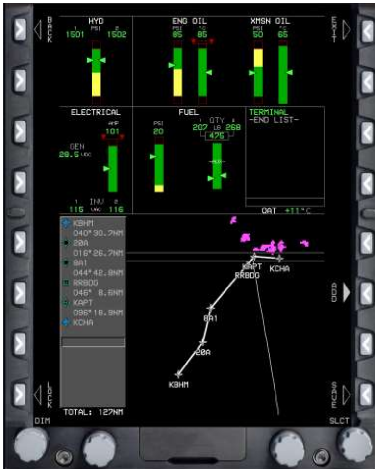
Figure 3-2 Example of Flight Plan on MFD
