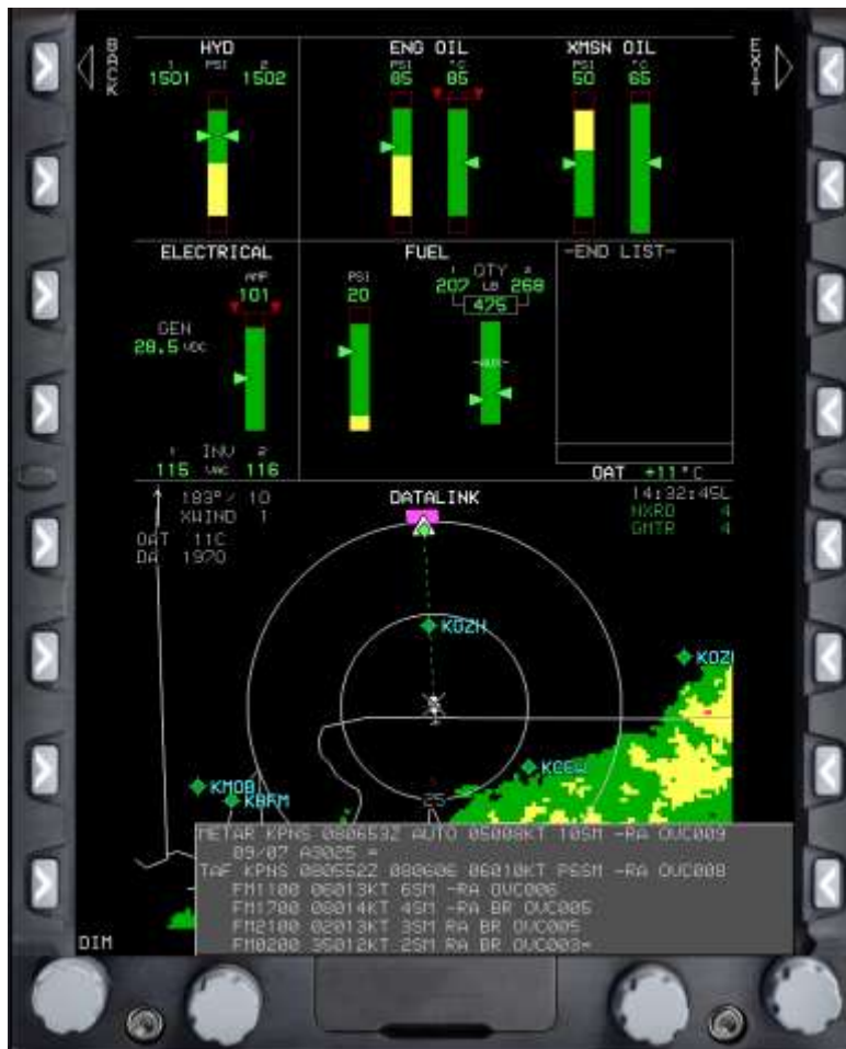
Figure 1-9 Expanded Airport METAR/TAF Text on MFD
