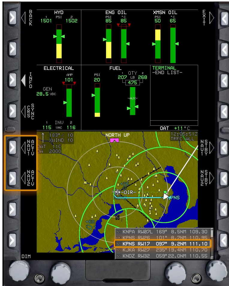
Figure 1-5 Setting Up an ILS Using the NRST Function
