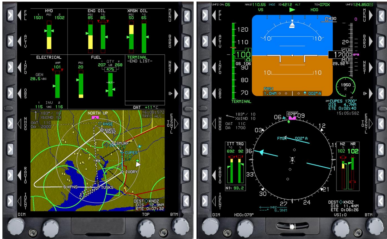
Figure 2-4 MFD and PFD Setup for KNDZ ILS Z 32 Approach with Active Leg from IVORY to CUPES
