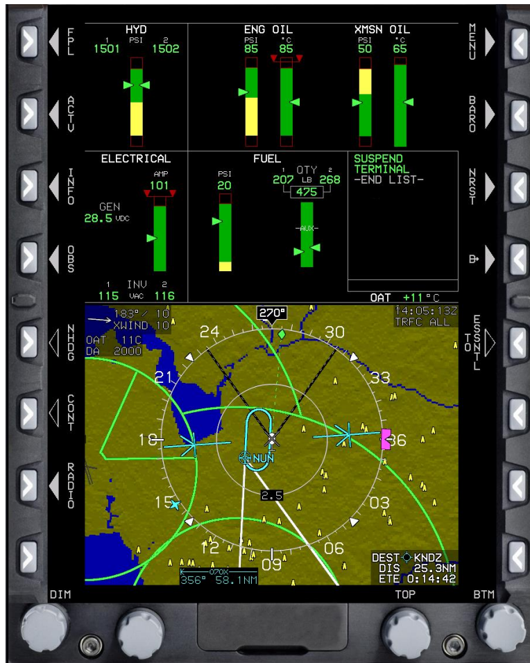
Figure 1-4 Suspended Waypoint Sequencing During a Holding Pattern
