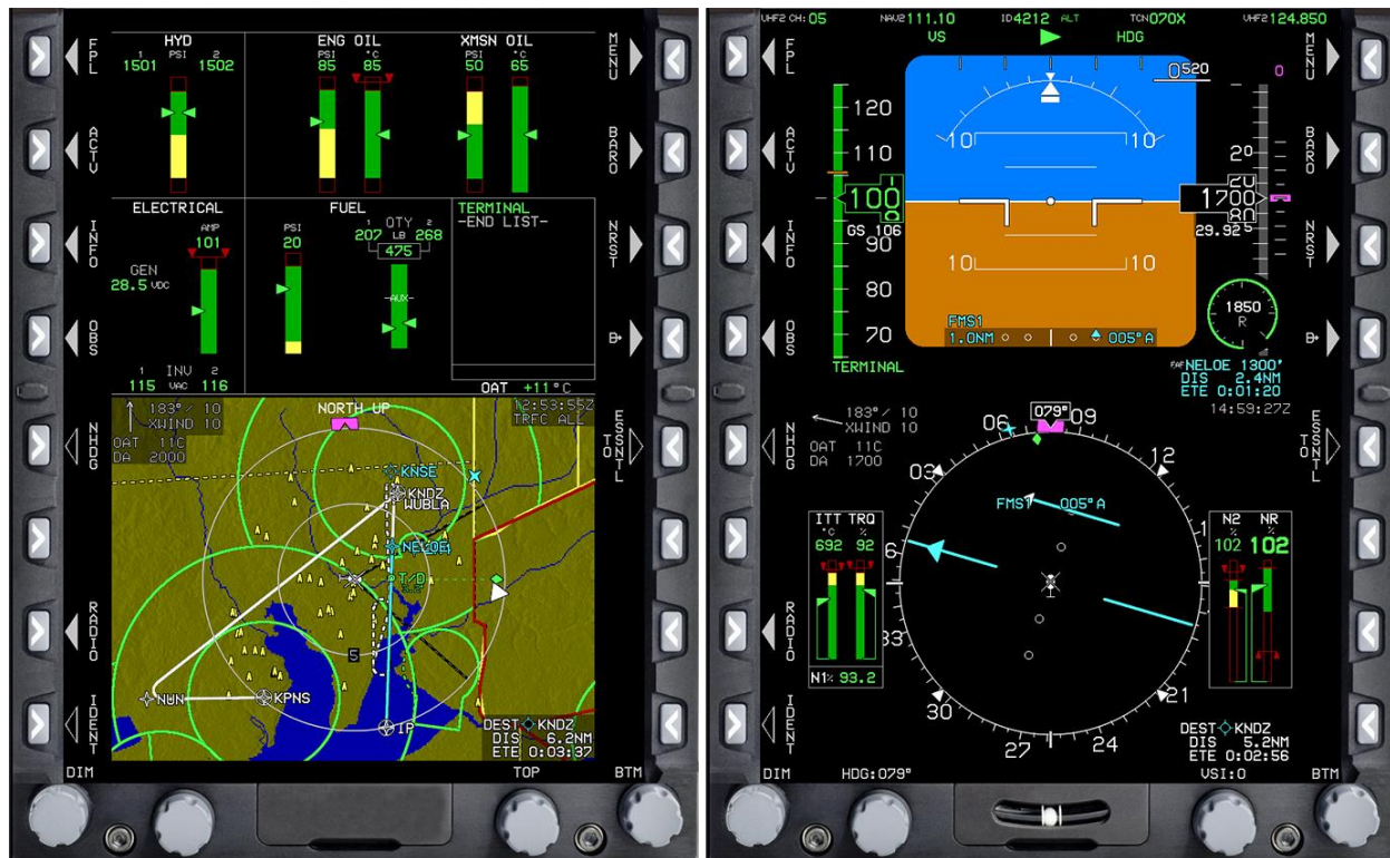
Figure 2-2 MFD and PFD Setup for KNDZ COPTER RNAV (GPS) 004 Approach
