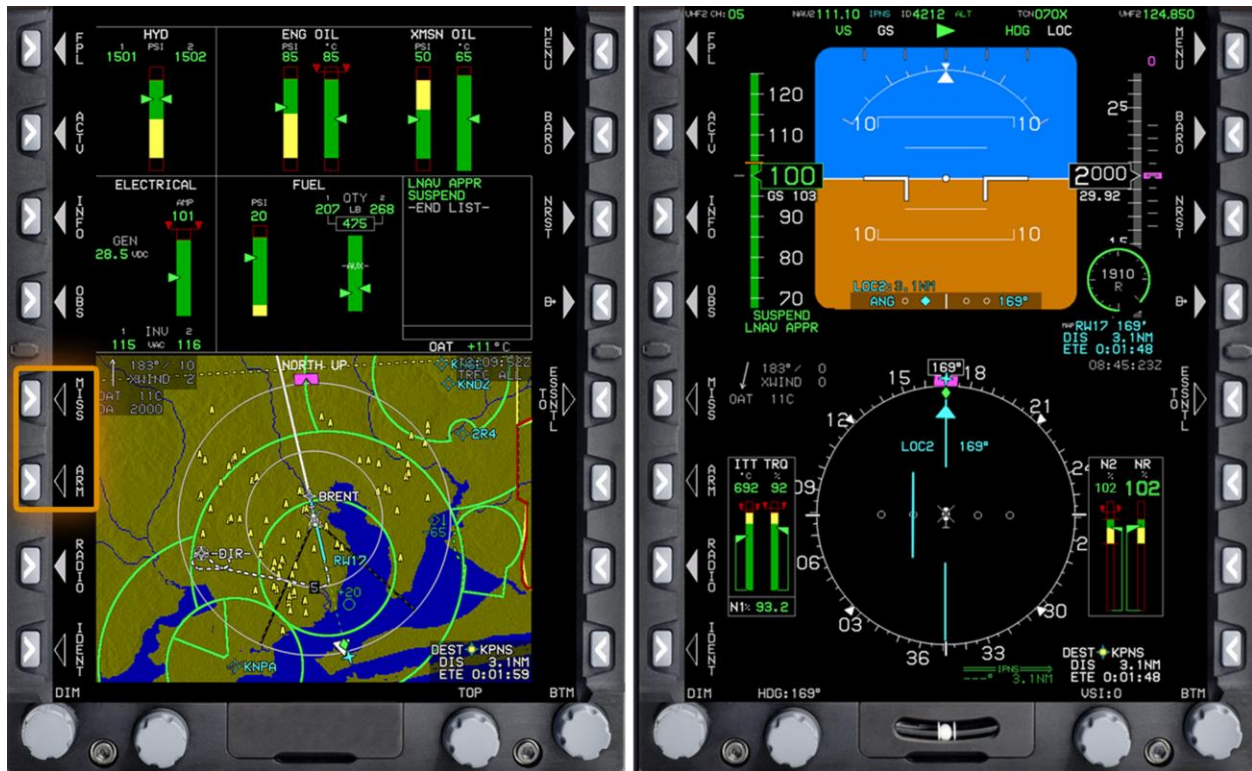
Figure 1-6 MFD and PFD Setup for the KPNS ILS RWY 17 Approach
