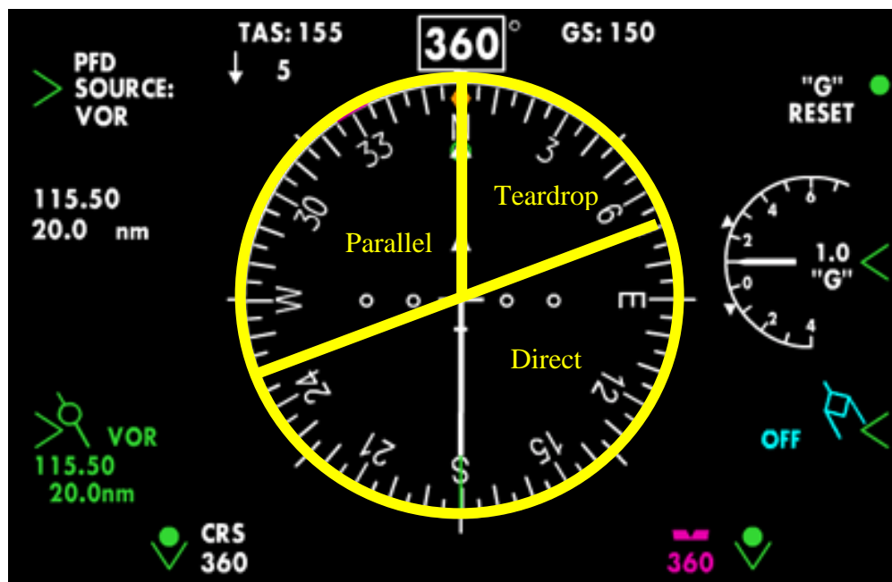
Figure 7-8 Standard Entry Diagram on HSI Display
