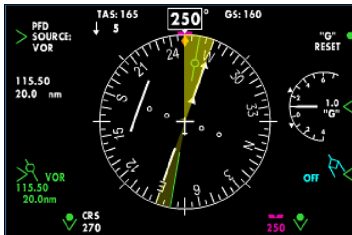
Figure 6-7 Double-the-Angle Intercept Inbound
