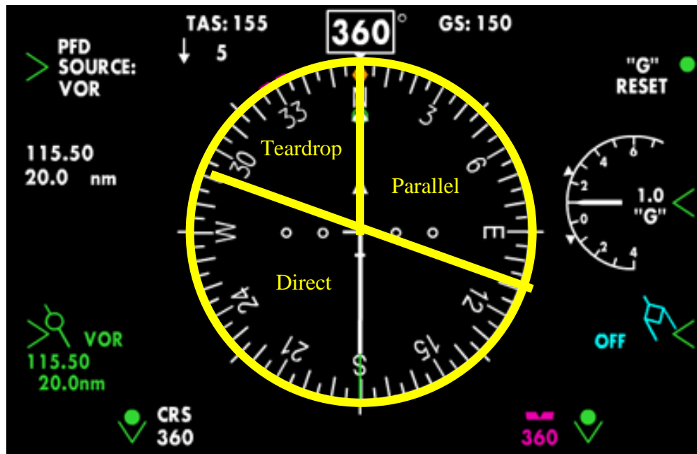
Figure 7-15 Non-Standard Entry Diagram on HSI Display
