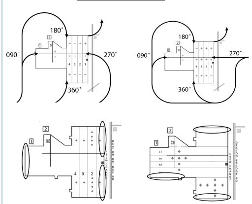
Channel 12 Field Elevation 159' MSL Max 11 aircraft, 4 per side, 3 sections max Max 2 aircraft on the Tactics side with T4002/3 active
