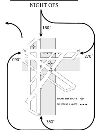
Channel 11, Field Elevation 150' MSL Night Max 6 aircraft, 3 aircraft per side. Primary unaided field for normal operations.
