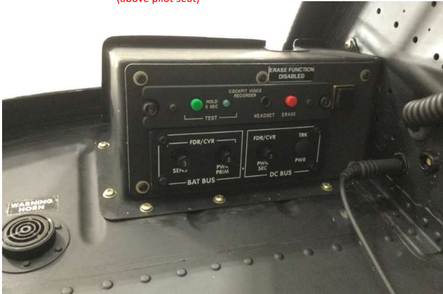
Cockpit Voice Recorder/Flight Data Recorder (above pilot seat)
