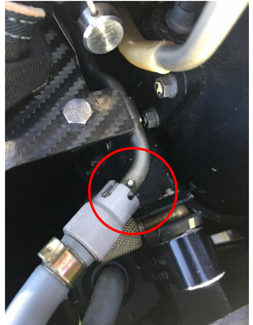
O2 Line Not Fully Installed
