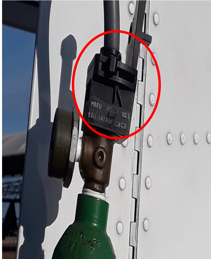
Transport Pin Still Installed
